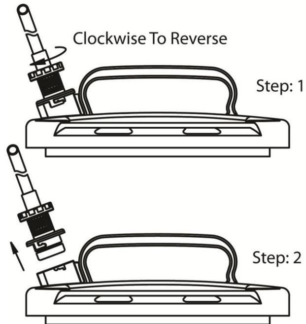
**CAUTION:** Be sure not to over-tilt, flooding safety valve. Container will not vent which will cause leakage and slow draining.
