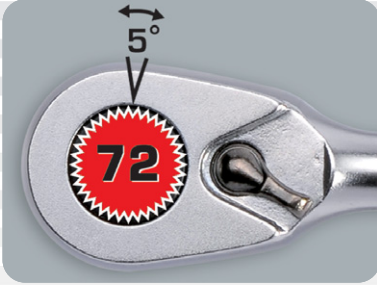
Extremely strong ratcheting mechanism with super fine toothing: 885 lb/in (100 Nm) 72 teeth, 5° ratcheting angle
